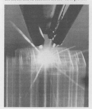
LENS FOCUS — Four nozzles deliver powder sintered by a laser beam into a Sandia thunderbird logo design.
